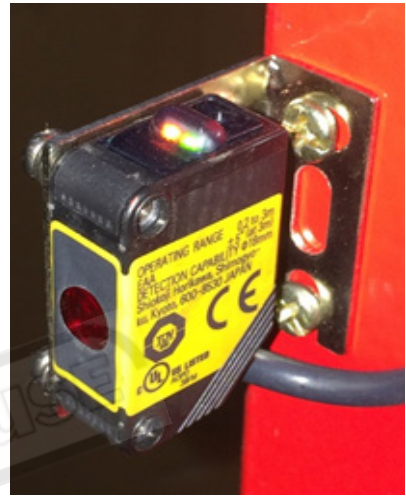
Has Power & aligned ok
